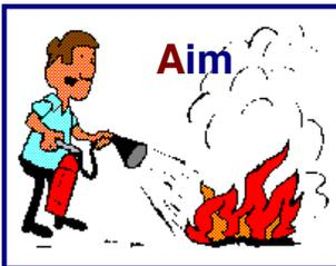
**Aim at the base of the fire.** If you aim at the flames (which is frequently the temptation), the extinguishing agent will fly right through and do no good. You want to hit the fuel.
